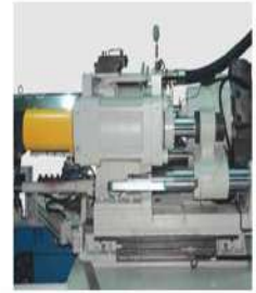
Oversized Mold Platen The stationary platen and moving platen are box-type structure. Increased sizes of mold platen significantly boosts structural strength.
